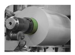
The **Hannecoil** rubber and polyurethane sleeves are recognized and used worldwide for their unique characteristics. Our mandrel sleeves are used to coil and uncoil rolled and coated steel and aluminium strip. At the same time they protect the sheet and ensure an excellent grip on the coil. Moreover, all our sleeves have outstanding expansion and shrinkage behaviour. Thanks to their elastic nature, they prevent scratches and marks on the strip.
